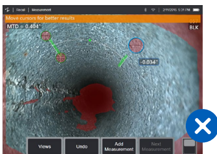
Incorrect cursor placement identified with 3D Point Cloud
